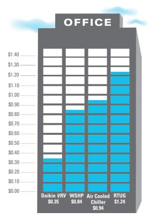
\*\* Modeled from a 3-story low-rise office building, 16,150 sq. ft./floor in Houston, TX. Costs to operate per square foot can vary based on regional climate, local utility provider and system design. Modeled in-house by PhD engineer using IES\_VE software according to ASHRAE 90.1-2010 in 2016.
